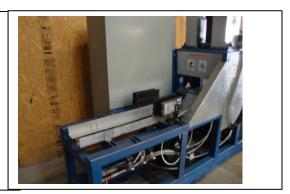
Hot Press System #HP100: This system comes as a standalone unit or may be connected to a conveyor dryer for auto pressing out of the dryer. One single die press 400 mm wide x 360 mm long. This system will accept one egg tray from 10 cell up to 18 cell, at a rate of up to 16 drops per minute or 960 trays per hour. This system comes complete with:
