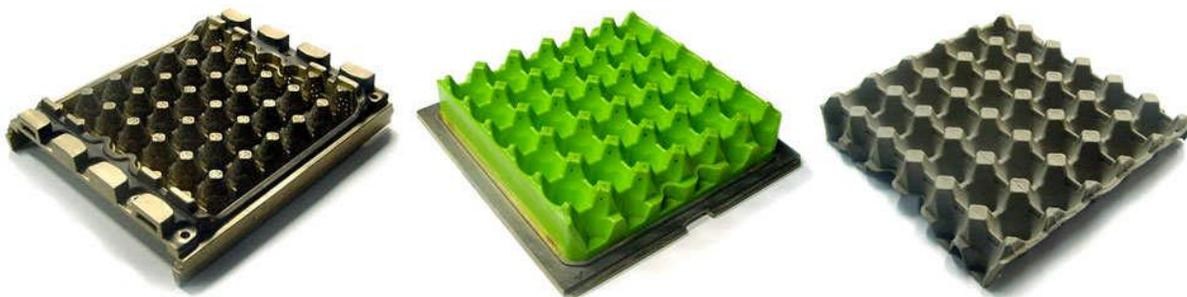
Two Aluminum moulding dies and two UHMW with aluminum base transfer dies included
